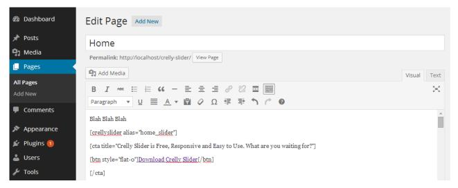
The second method is using a php function. Write <?php if(function\_exists('crellySlider')) crellySlider('your\_slider\_alias'); ?>. Put the function wherever you want in a theme php file (e.g. index.php).
